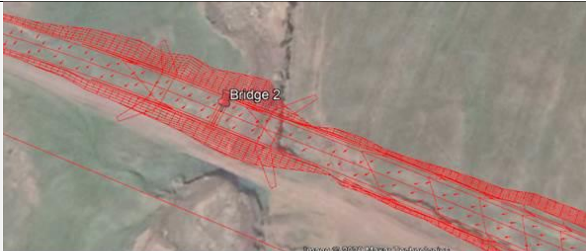
Figure 1-4: Bridge 2 - new bridge proposed to be constructed across the Mjanyana River roughly 50m to the right of the existing bridge.
