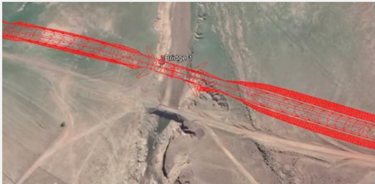
Figure 1.3: Bridge 1 - new bridge proposed to be constructed across the Tora River roughly 50m to the right of the existing bridge.
