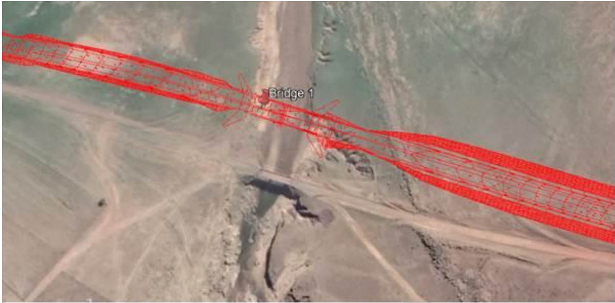
Figure 2-3: Bridge 1 - new bridge proposed to be constructed across the Tora River roughly 50m to the right of the existing bridge.
