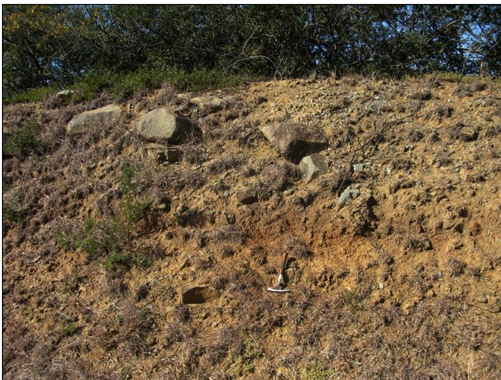
Fig. 28. Poorly-sorted, bouldery colluvial gravels – mainly sandstone, with occasional dolerite clasts - overlying Balfour Formation saprolite (Hammer = 30 cm) (Loc. 299).
