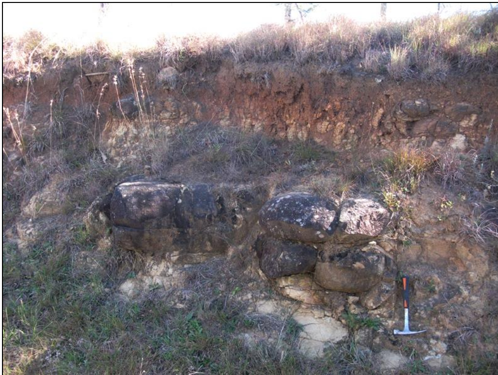
Fig. 15. In situ , subrounded corestones within a deeply-weathered sandstone package overlain by crumbly sandstone saprolite and orange-brown gravelly soils (Hammer = 30 cm) (Loc. 298).
