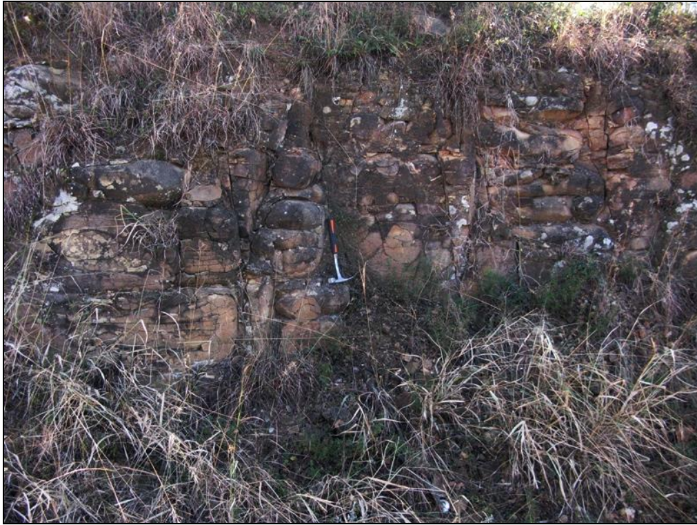
Fig. 14. Well-jointed channel sandstone in road cutting showing typical dark brown weathering patina, open joints and incipient corestone formation (Hammer = 30 cm) (Loc. 298).
