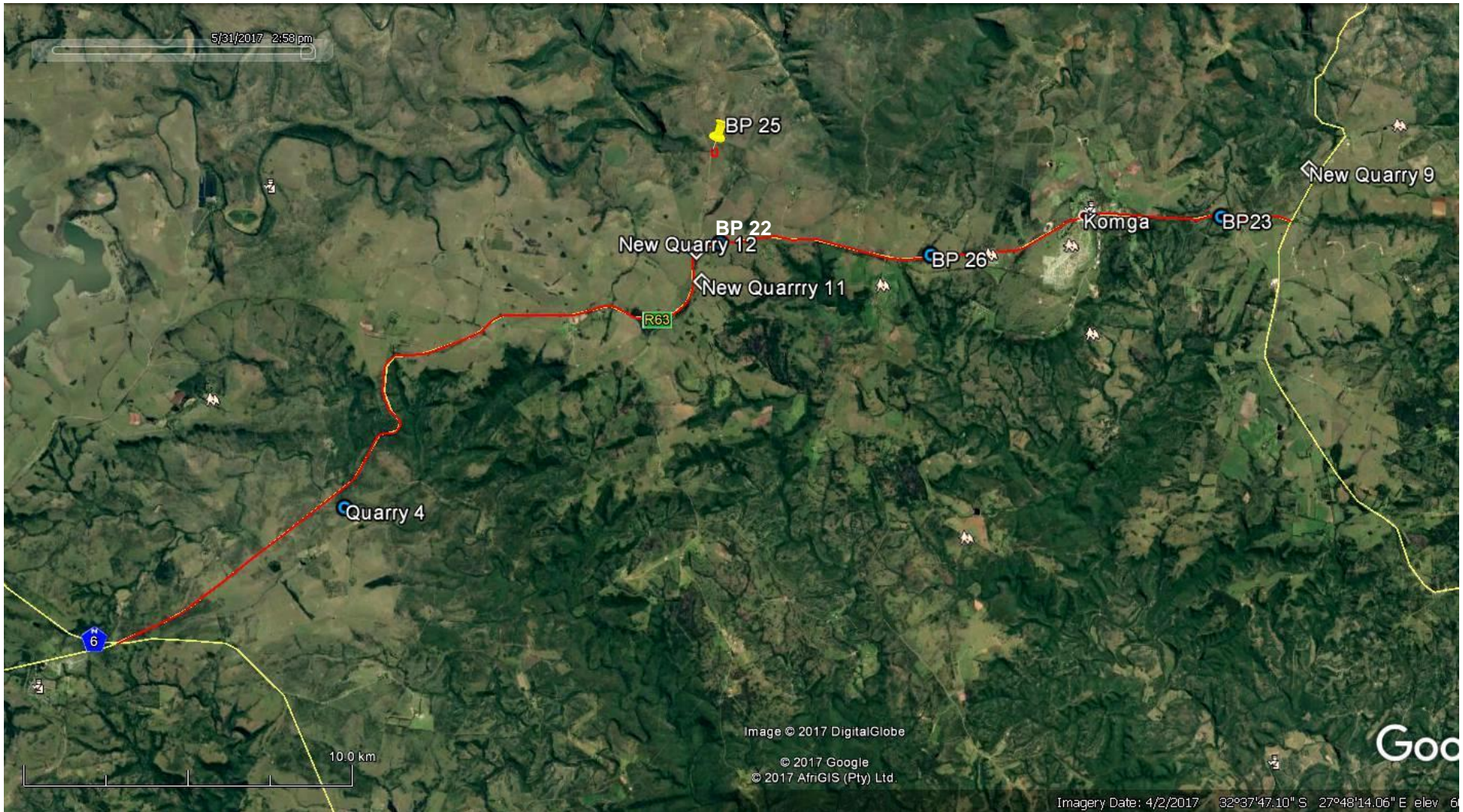
Fig. 2. Google earth© satellite image of the R63 Section 16 study area (red line) between the N6 and the N2 near Komga, Eastern Cape. The eight proposed borrow pits and quarries associated with the road upgrade are also indicated (See Table 1). Quarries 11 and 12 and Borrow Pits 22 and 25 are excavated into Karoo dolerite while the remaining sites are excavated into Late Permian sedimentary rocks of the Balfour Formation (Lower Beaufort Group).
