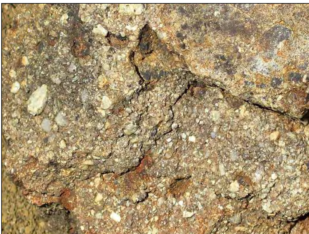
Figure 26. Close-up of immature, gritty, feldspathic Normandien channel sandstone facies seen above showing kaolinitised feldspar clasts up to 1 cm long.
