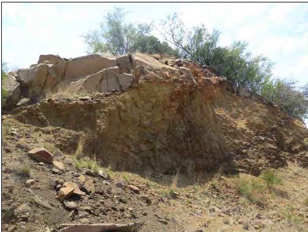
Figure 33. Cut face in existing quarry, BP25 study area showing deeply-weathered massive dolerite ( sabunga ) cut by an inclined dolerite dyke with fresher dolerite at surface.
