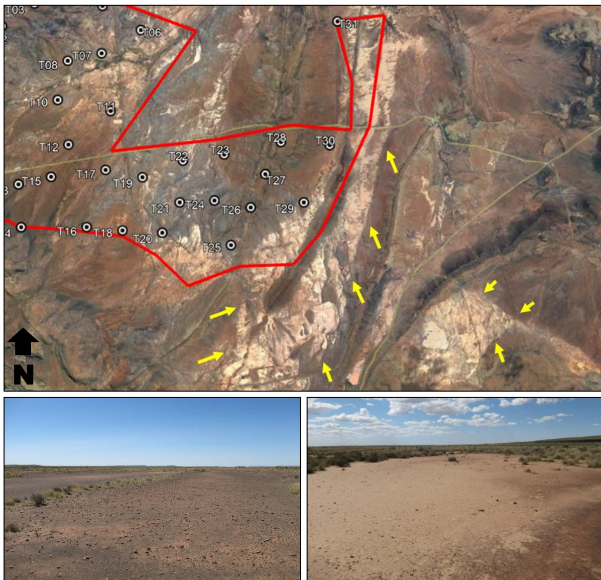
Figure 12: (Top) Digital satellite imagery depicting broad areas of increased clay content hosting episodic preferential flow paths (yellow arrows), in relation to the eastern portion of the study area (red outline) and associated turbines. (Bottom) Photographs of these areas of episodic preferential flow paths.
