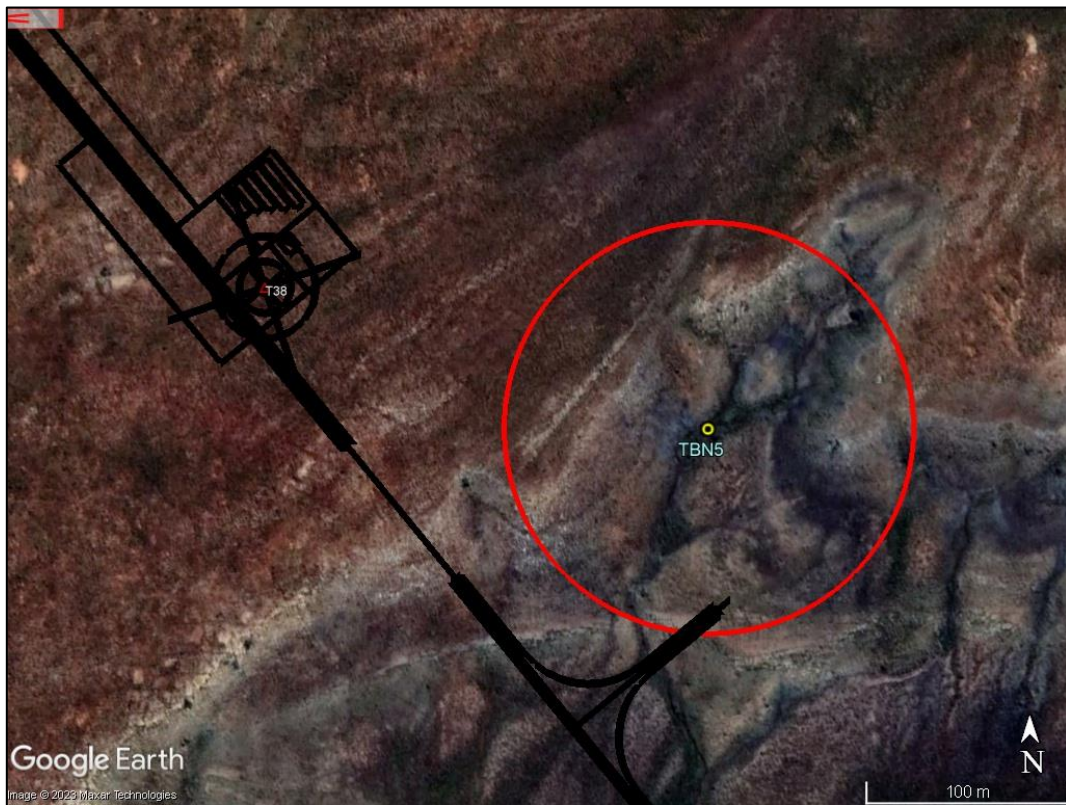
Figure 10-2: Aerial image indicating the 100m no-go development buffer recommended for site TBN05 in relation to project infrastructure components.
